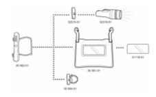
The Divator Rail System is quickly and easily attached to the Divator Full face mask making it possible to attach various accessories to the mask. It can, for example, hold a welding visor frame, dive lights, a video camera, video lights or sonar heads.
