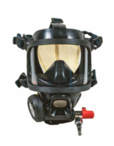
When donning the first breath version of the S-USA mask it will automatically activate when the user inhales to take the first breath. A handle on the breathing valve is used to shut it off when the mask is removed.
