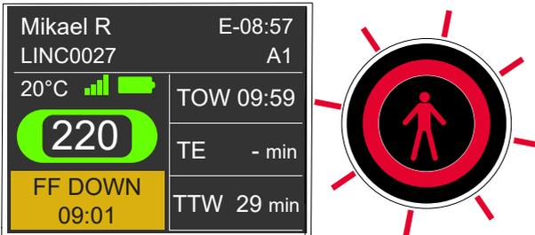
3. If an emergency team is deployed and pushes in the rescue tally key in the affected BA set: The warning in the FF display will change to green 'ADSU RESET' and the FF button will stop blinking red.
