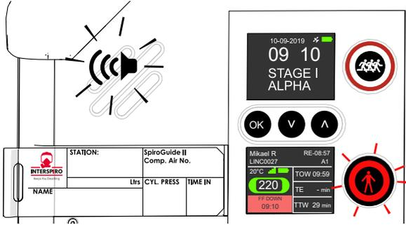
2. The ECO can acknowledge the alarm by pressing the FF button. The sound will stop and the colour on the warning in the FF display will change to amber.
