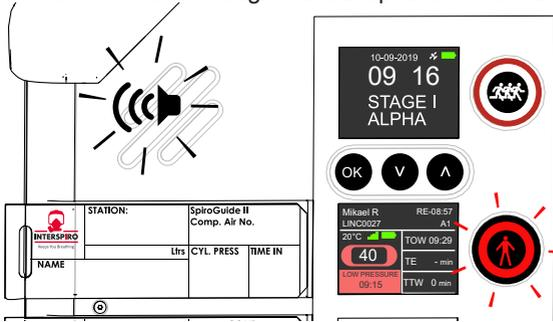
5. The ECO can acknowledge the alarm by pressing the FF button. The sound will stop and the colour on the warning in the FF display will change to amber.
