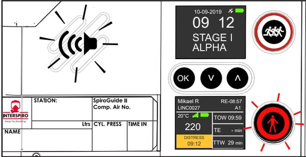
2. If an emergency team is deployed and pushes in the tally key in the firefighter's DDU, the sound will stop, the FF button will stop blinking red and the warning in the FF display will change.
