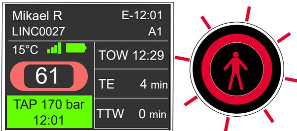
6. If an emergency team is deployed and inserts a rescue tally key into the affected wearer's DDU, the warning in the FF display will change to green.
