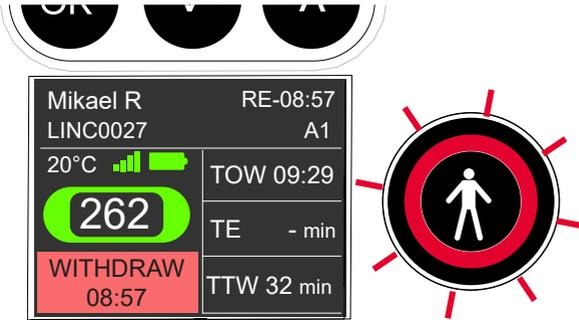
3. The BA wearer acknowledges the Withdraw signal by pressing the black button on the DDU.
